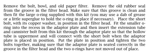
Tighten the two bolts but do not over-tighten. You are now ready to fit a spin-on filter to your Vauxhall Velox.
